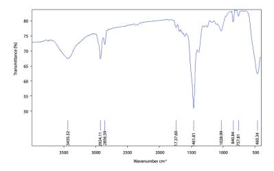
$\textbf{Figure 1.} \ \textbf{FTIR} \ spectrum \ of \ synthesized \ ZnO$
